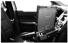
The pilot program testing was comprised of a bench test for form factor ID and the second phase was in-car testing. Getac's V110 was suggested due to its lightweight design, 7th generation Intel processors and sunlight-readable large 11.6" display.
